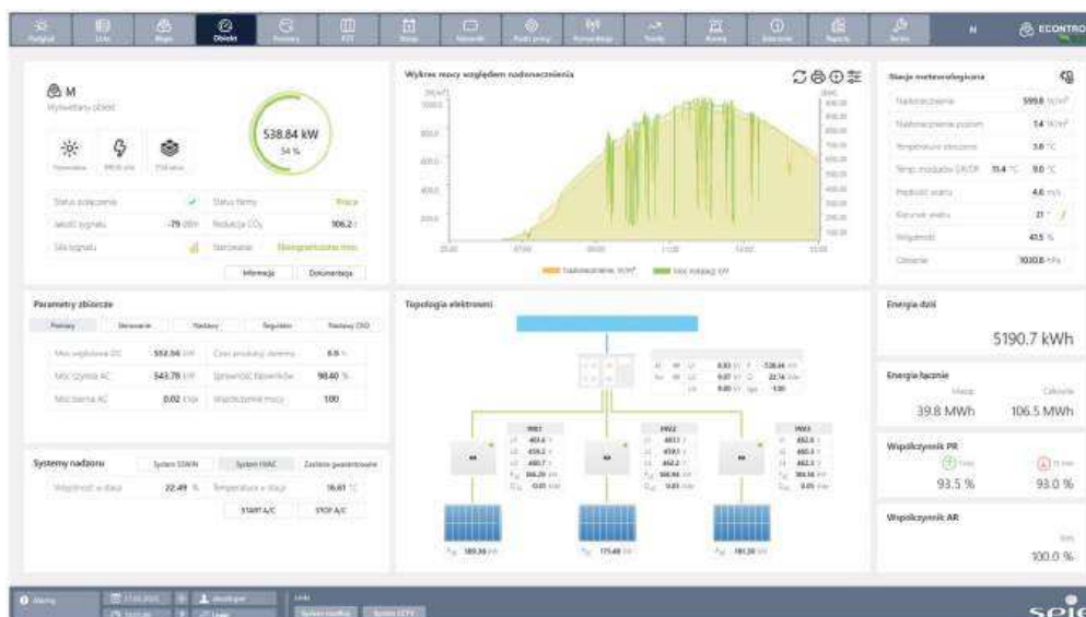
Rys. 3. System ECONTROLoze – Farma PV
